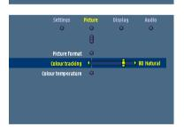
Adjustments are generally made by setting an on screen slider to the required value. For this use Cursor Control left/right. Confirm the adjustment by pressing OK.
